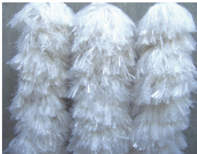
Fig. 2. Picture of fiber polypropylene media used for this study (color figure available online).
